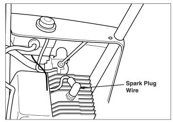
Figure 16. Servicing Spark Plug
